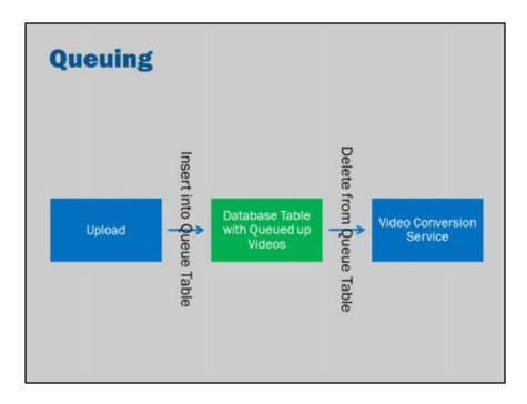
A simple approach to building a queue would be to insert a task into a database table during from one process (e.g., after upload).
