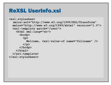
Then ReXSL would transform the XML output of the JAX-RS API into a HTML document.
