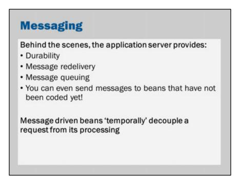
**Durability**: Once accepted, a message will not get lost when the Java EE server stops or loses power suddenly. It is only removed from the queues once it has been successfully processed.
