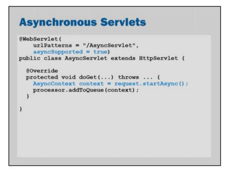
To use asynchrony in servlets, just add asyncSupported = true to the @WebServlet annotation.
