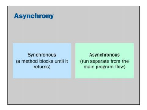
In computer programming synchronous means that your code is executed within the ordinary flow of control.
