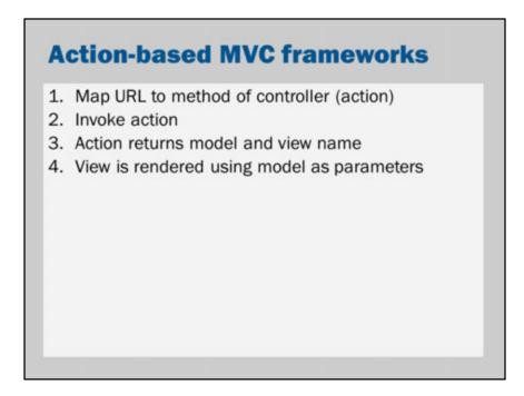
Action-based MVC frameworks typically follow the four steps listed in the slide.
