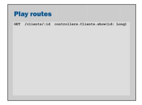
The mapping between URLs and the controllers/actions is not achieved with annotations. Instead a route mapping file is used to configure the mappings.
